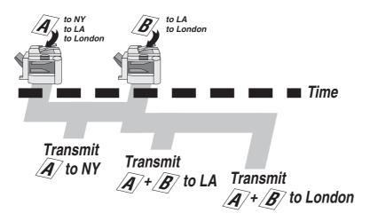
During memory transmission, this machine searches its memory for reserved files (up to 5 files) to transmit to the same destination, automatically batching, and transmitting them in a single phone call.
